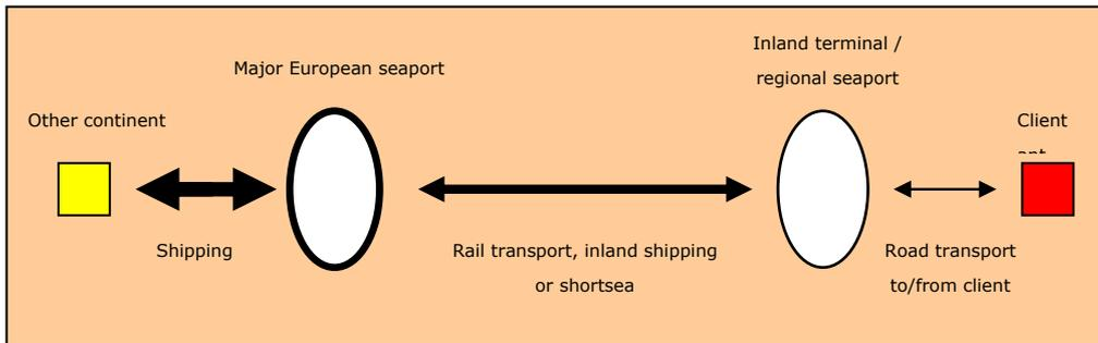
Figure 4.3 Diagram of an intermodal transport chain
